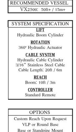
Base or Standpipe Mount 360° Manual Rotation 12 / 24V DC Power Wireless Remote
